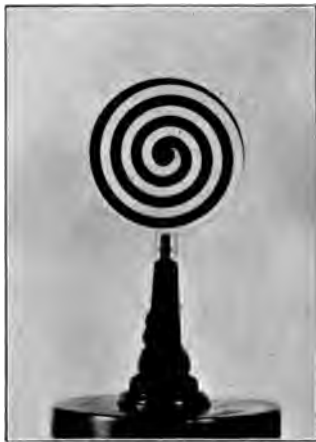
FIG. 12. — Apparatus for producing an after-image of motion, in direction the reverse of the original movement.
